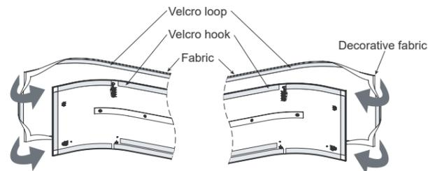
4. Insert the fabric into the top and bottom side of the air inlet grille. Attach the hook and loop of velcro tape fully together. As shown on figure as below.
