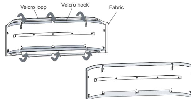
5. Reassembly the air inlet grille by reverse process of 1.
